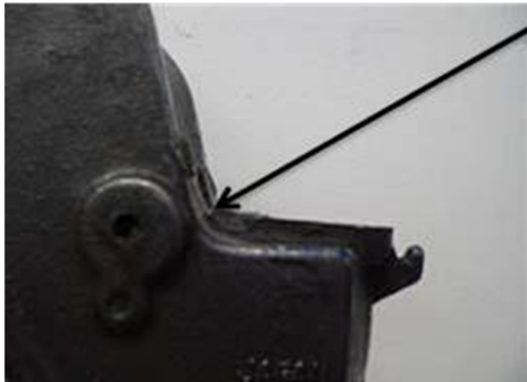
Photo 3: Steering bracket with the turning stop removed
