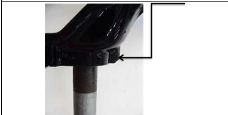
Photo 2: Steering bracket with centre turning lug removed
